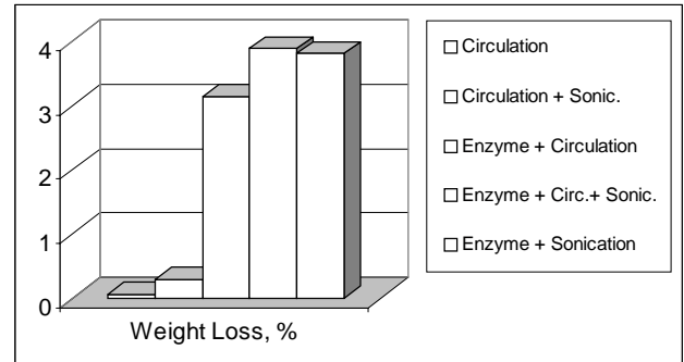
Figure 3. Effect of the treatment conditions on weight loss of cotton printcloth in Test #2.
