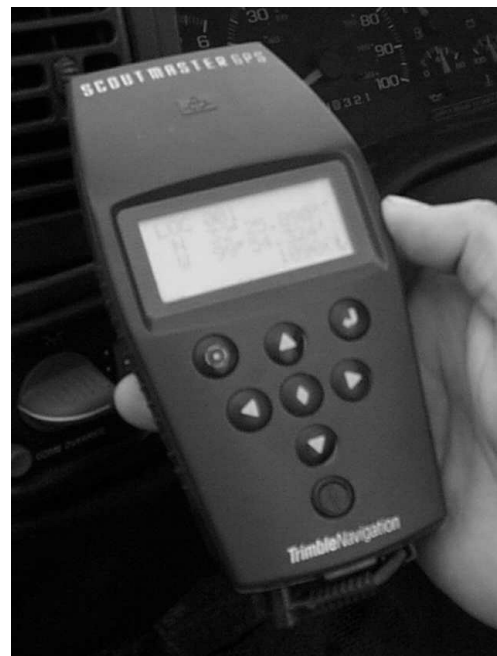
Figure 1. Scout Master Hand-held Global Positioning System Unit (Trimble Navigation).
