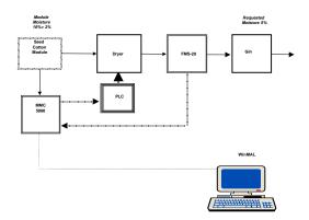
Assuming that the seed cotton module moisture level is 10%, in order to lower the moisture at the entrance to the gin stand to 5%, the cotton should be dried by 5%. Since the moisture level of the seed cotton m o d u l e, m e a s u r e d b y resistance/capacitance moisture indicators is known with an accuracy of 2%, the cotton is dried by additional safety margins of 20%.
