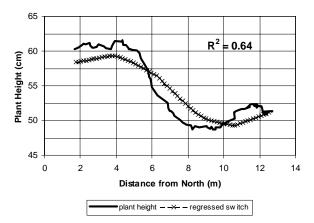
Figure 7. Graph of 31-reading moving average of plant height values and predicted heights from multi variate regression of switch data. Values at beginning and end of shown lines reflect influence of full data set instead of only plot 4 from midday June 11, 1998.
