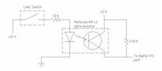
Figure 2. Schematic diagram of circuit used for logging of switch data on cotton height sensor.
