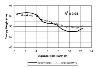
Figure 4. Graph of 9-reading moving average of canopy height values and predicted heights from multi variate regression of MAC data. Values at beginning and end of shown lines reflect influence of full data set instead of just plot 4 from June 11, 1998, midday.
