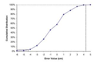
Figure 10. Cumulative distribution of errors in predicted canopy height from switch output for 10 plots from midday June 11 and 1 plot from afternoon July 16, 1998.
