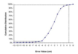
Figure 9. Cumulative distribution of errors in predicted plant height from switch output for 10 plots from midday June 11 and 1 plot from afternoon July 16, 1998.
