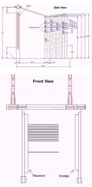
Figure 1. Side and front views of cotton height sensor. Side view shows infrared sensors (MAC) on left side and switch bank on the right. Dimensions shown in centimeters.
