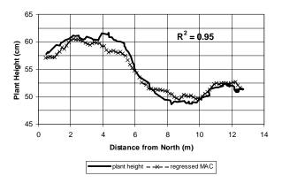
Figure 3. Graph of 31-reading moving average of plant height values and predicted heights from multi variate regression of MAC data. Values at beginning and end of shown lines reflect influence of full data set instead of just plot 4 from June 11, 1998, midday.
