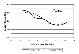
Figure 8. Graph of 9-reading moving average of canopy height values and predicted heights from multi variate regression of switch data. Values at beginning and end of shown lines reflect influence of full data set instead of only plot 4 from midday June 11, 1998.
