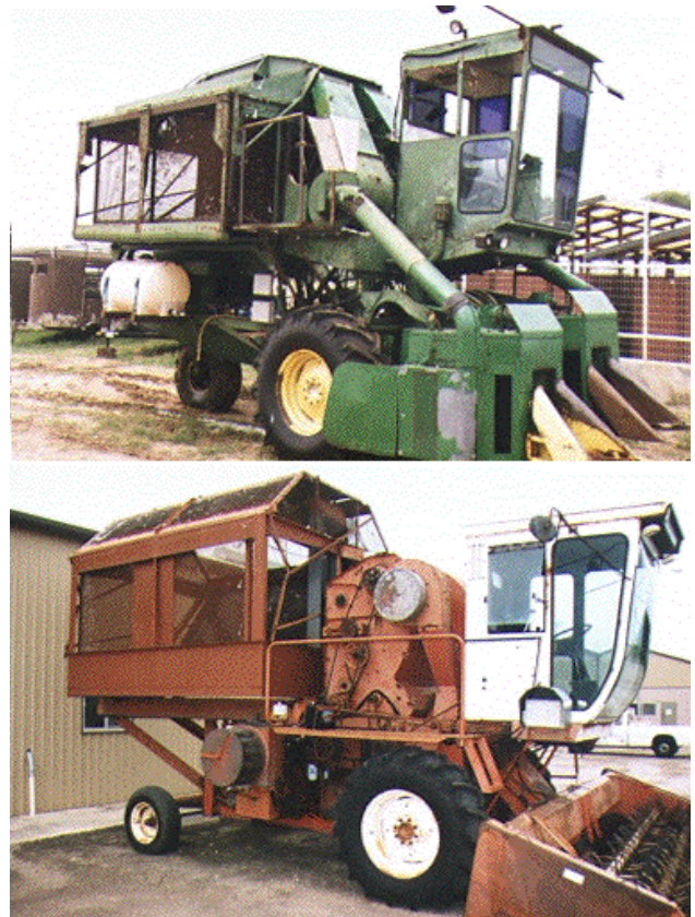
Figure 1. John Deere 299 cotton picker (top) and Allis Chalmers 860 broadcast-header stripper (bottom) modified with computerized system for direct measurement of seedcotton yield.
