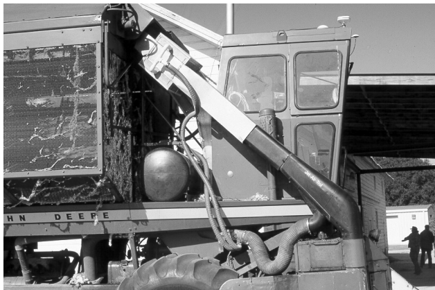
Figure 2. AirBox enclosure mounted on picker. Note air supply lines from fan to AirBox.
