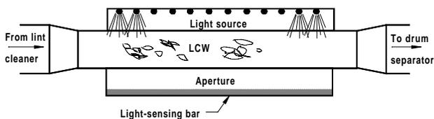
Figure 1. Diagram of light-sensing bar/duct configuration for small research gin (Study 1).
