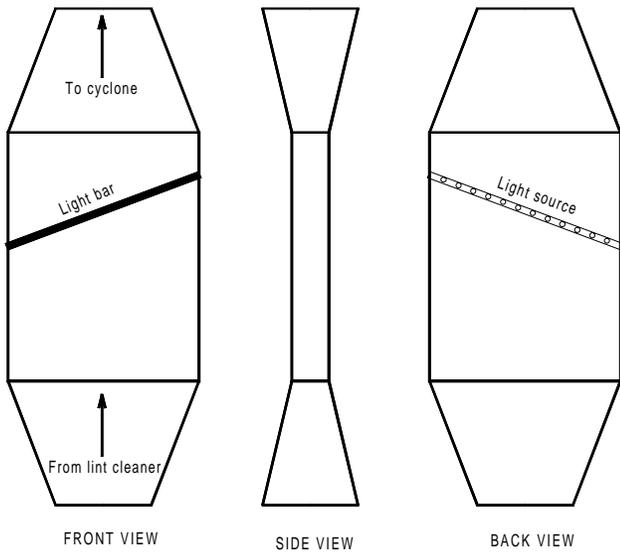
Figure 5. Diagram of light-sensing bar/duct configuration for full-size gin (Study 2).
