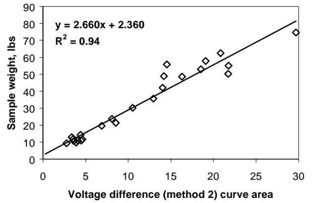
Figure 7. Sample weight vs. Voltage difference (method 2) curve area for data from full-size gin (Study 2).
