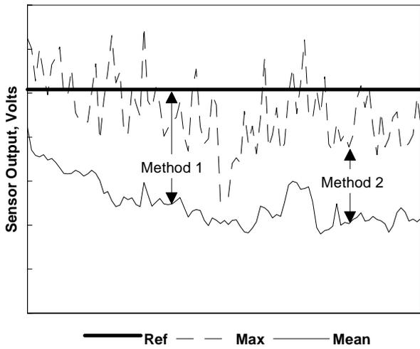
Figure 6. Example voltage difference calculation by method 1 (difference from the reference) and method 2 (difference from the maximum).
