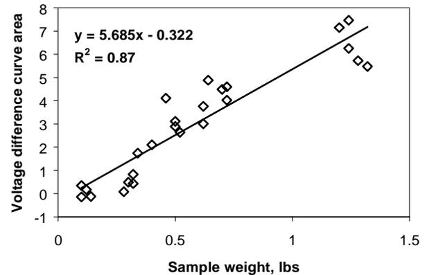
Figure 4. Voltage difference curve area vs. Actual flow-rate for data from small research gin (Study 1).
