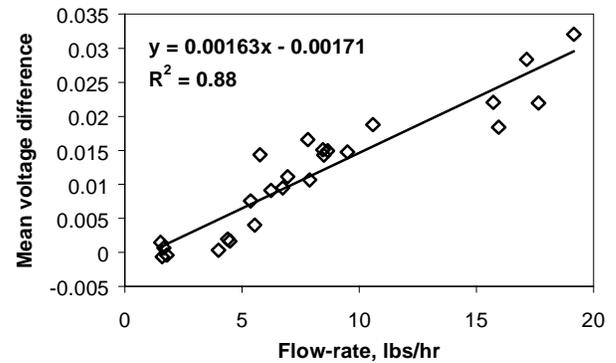
Figure 3. Mean voltage difference vs. Actual flow-rate for data from small research gin (Study 1).
