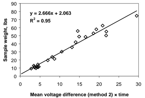
Figure 8. Sample weight vs. Mean voltage difference (method 2) X time for data from full-size gin (Study 2).
