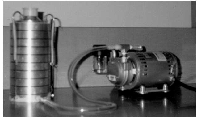
Figure 1a. The Graseby Anderson Cascade Impactor (left) and pump.
