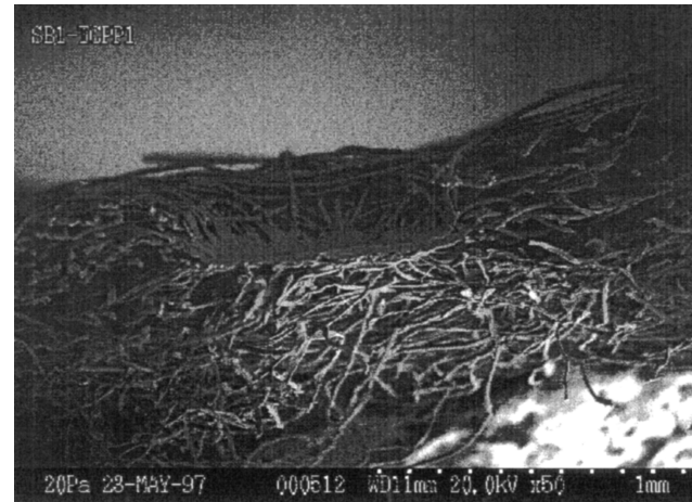
Figure 2. Cross-Sectional SEM photograph of Laminate, Sample #1 (SB1-TCPP1)
