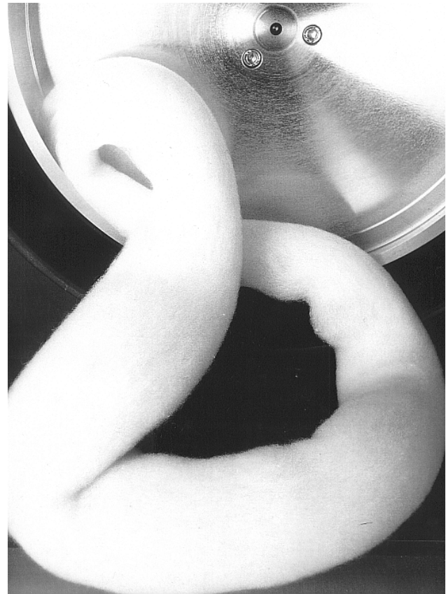
Figure 11. Rotor of MDTA 3 with fibre ring
