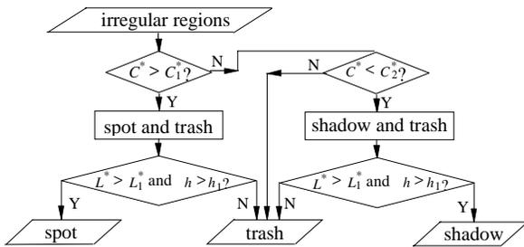
Figure 6 Multi-Dimension Thresholding
