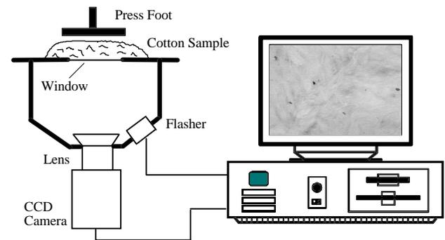
Figure 1 Schematic Set-up of the System
