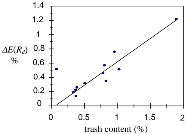
Figure 12 Relationship between  $\Delta E(R_d)$  and Trash Content
