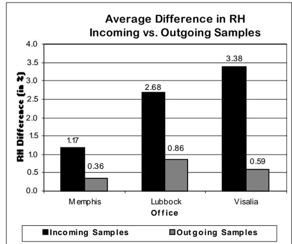
Figure 2. Average difference in RH readings for incoming vs. outgoing probes (all study data).
