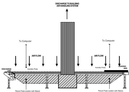
Figure 1. Side View of RCU including study set-up.
