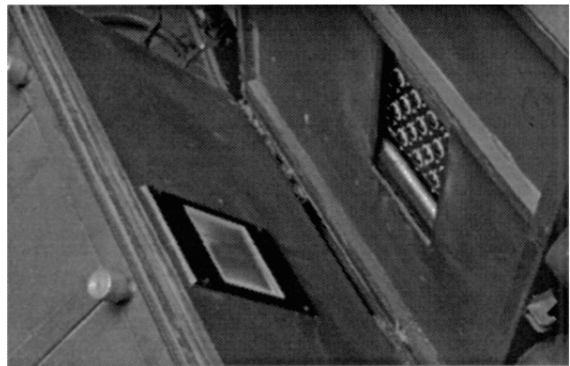
Figure 2. Paddle sampler in closed position with the color/trash measurement head moved away to show detail.
