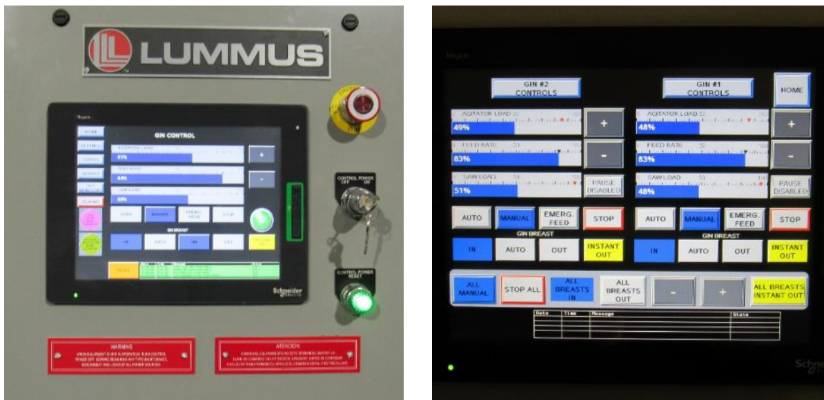
Figure 10. DGC 2020 Digital Gin/Feeder Controls Operator Interface at the gin stand (left) and Remote Gin/Feeder Controls Interface, located in the Main Gin Controls Console (right).
