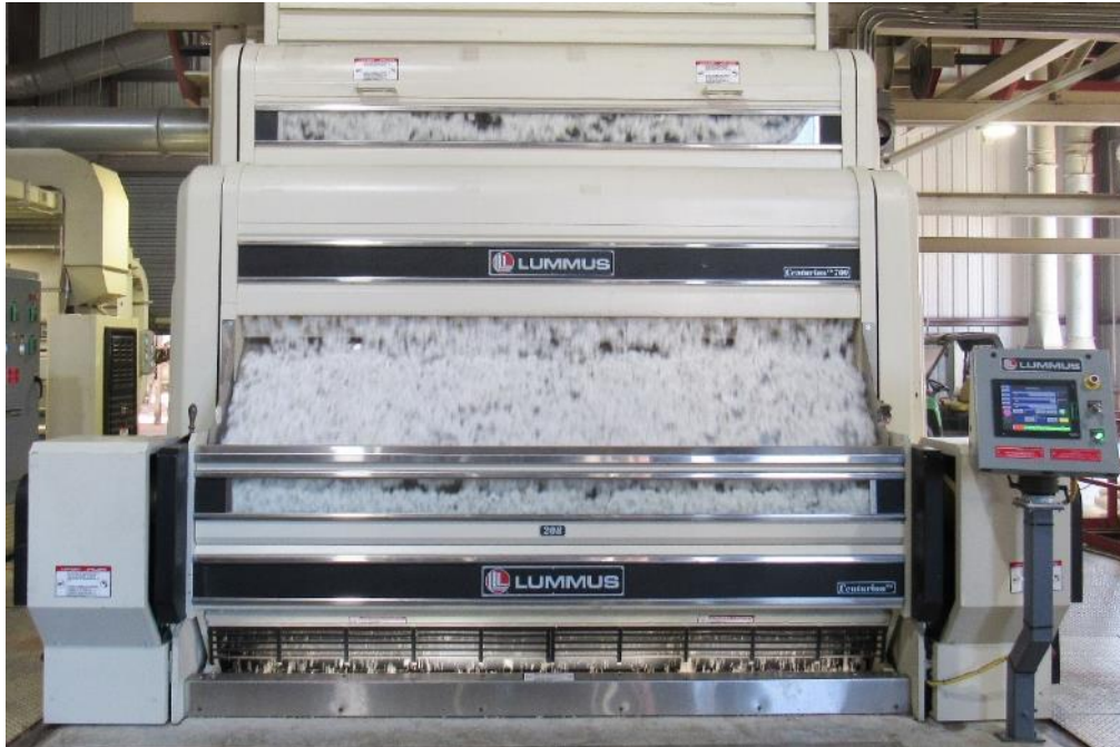
Figure 9. 10' Centurion™ 700 Feeder over 208-Saw Centurion™ Gin.
