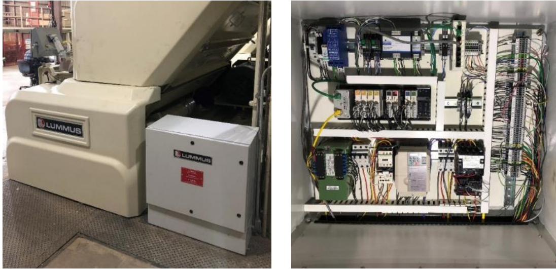
Figure 2. DGC 2020 Digital Gin/Feeder Controls (Complete Conversion).
