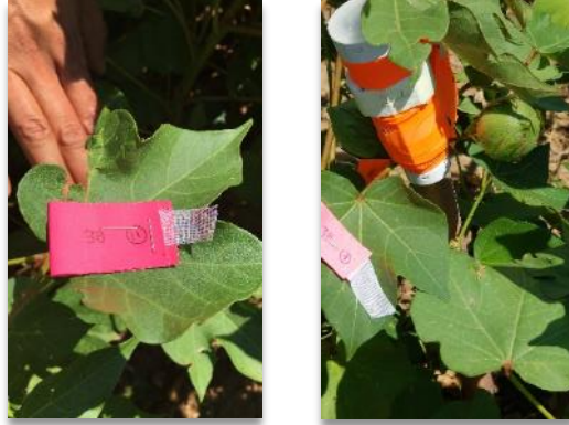
Figure 2. Left: Fabric with sentinel H. zea eggs placed on a cotton leaf. Right: Hobo temperature and relative humidity datalogger in canopy near fabric with sentinel H. zea eggs.
