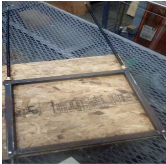
Figure. 7. Brush frame and lead screw assembly.
