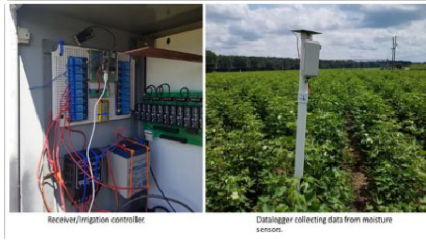
Figure 4. Receiver/controller installed on the lateral mover irrigation system, and the dataloggers collecting data from moisture sensors installed at the center of each of the sixteen plots.
