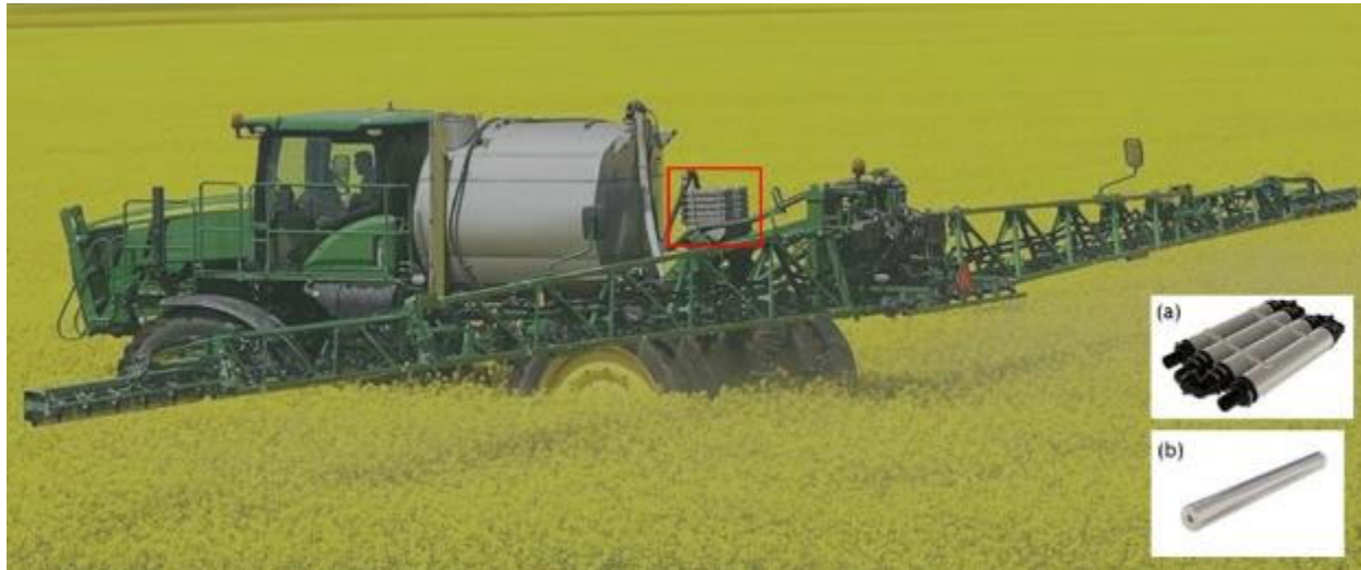
Figure 1. MagGrow technology installed on a boom sprayer. (a) Manifold and (b) stainless steel encased magnetic rods (Image source: www.maggrow.com ).
