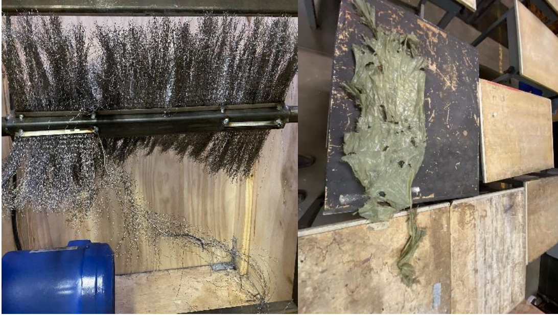
Figure 6. Failed brush assembly (a) and removed plastic (b).
