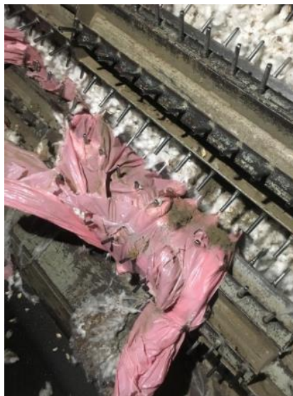
Figure 1. Module wrap on module feeder dispersing cylinder.
