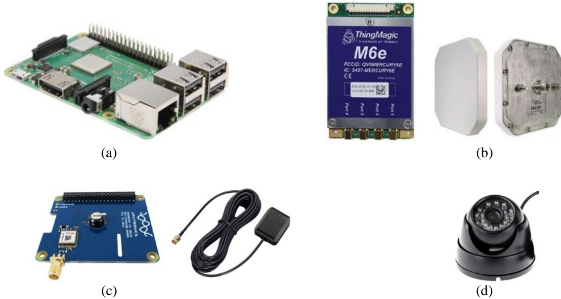
Figure 1. The smart cotton module tracking system contains (a) data logging CPU, (b) RFID module, (c) GNSS module, and (d) cameras.
