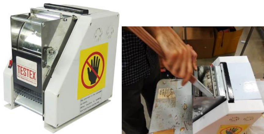
Figure 1. A tabletop gin which is being used while lab tests.
