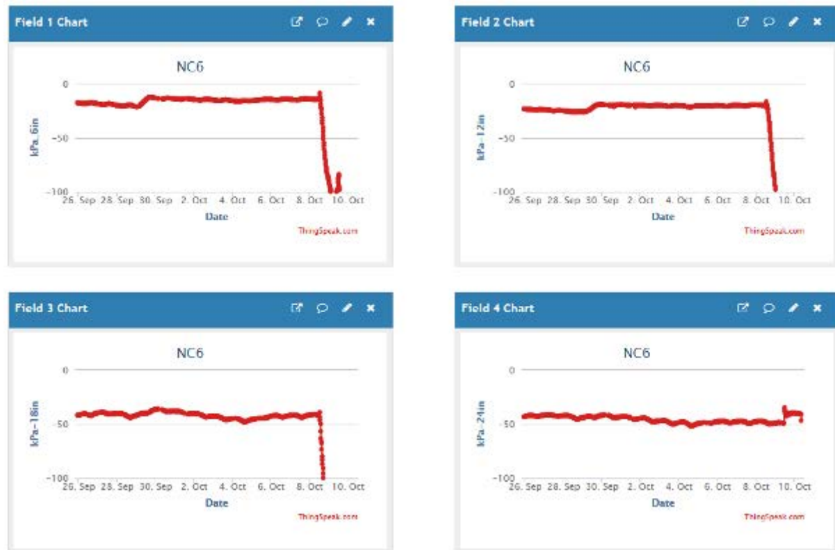
Figure 2. Soil moisture from four sensors installed in one of the cotton plots (plot #6).
