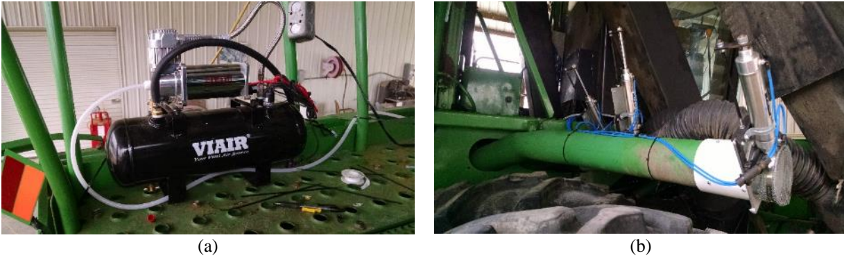
Figure 10. Air compressor for supplying air to the pneumatic control circuit, as installed (a), and view from the right side of the picker (b), showing two blast gates (left) for controlling airflow to the outer two picking heads on the right side of the picker and one blast gate (right) for controlling exhaust air. Note in image that the blast gate for the exhaust air is closed and the blast gates for the picking air are open.
