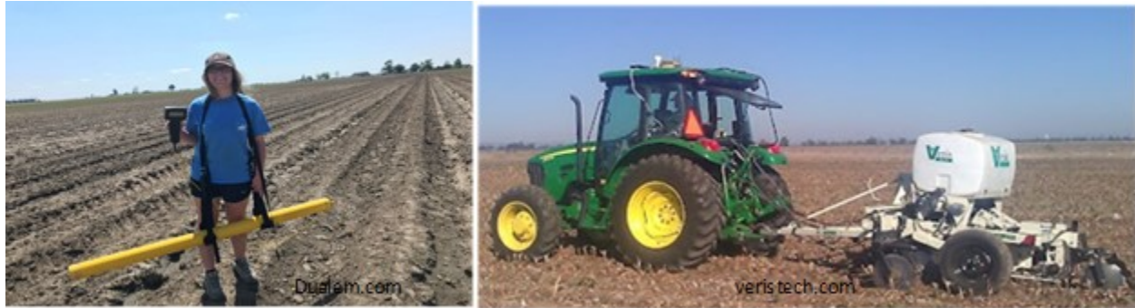
Figure 3. Sample points for different soil textures were set after cotton planting using a non-invasive DUALEM-1H (left). Classification of soil textures for yield analysis were made following harvest using a Veris Soil Surveyor (right).
