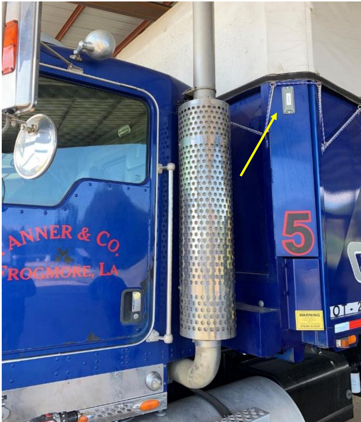
Figure 7. Truck RFID tag mounted on the front driver's side corner of the bed.
