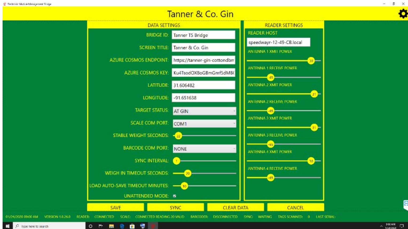
Figure 9. RFID Scale Bridge software settings page accessed by clicking the gear icon in the upper right corner of the home screen (figure 7).
