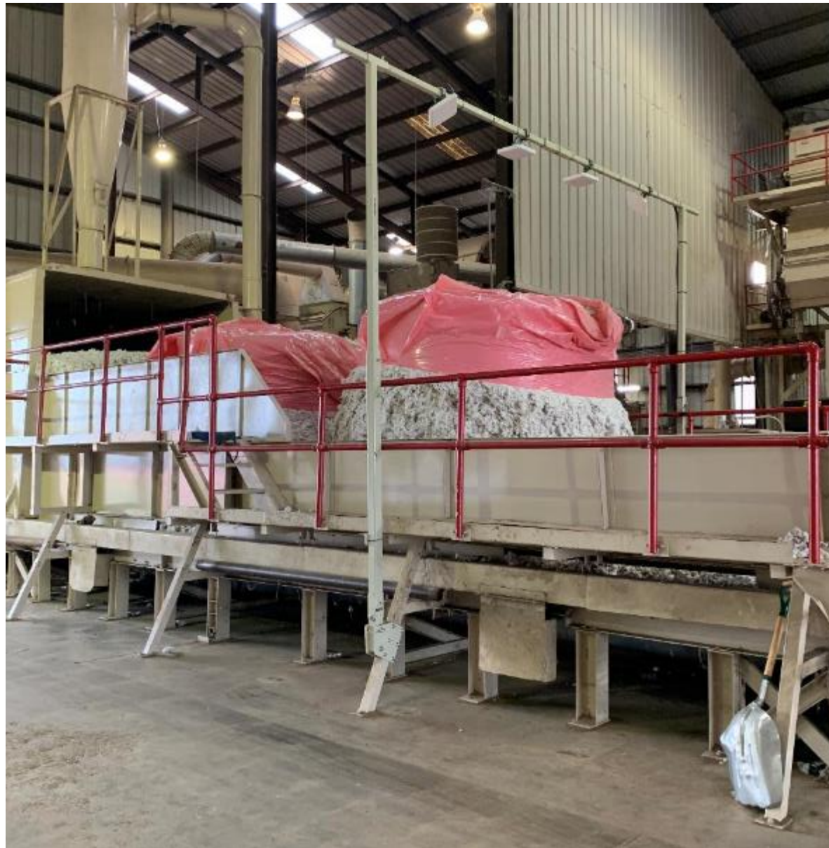
Figure 12. RFID scanning system mounted above the roller bed of the module feeder at Tanner and Co. Gin.
