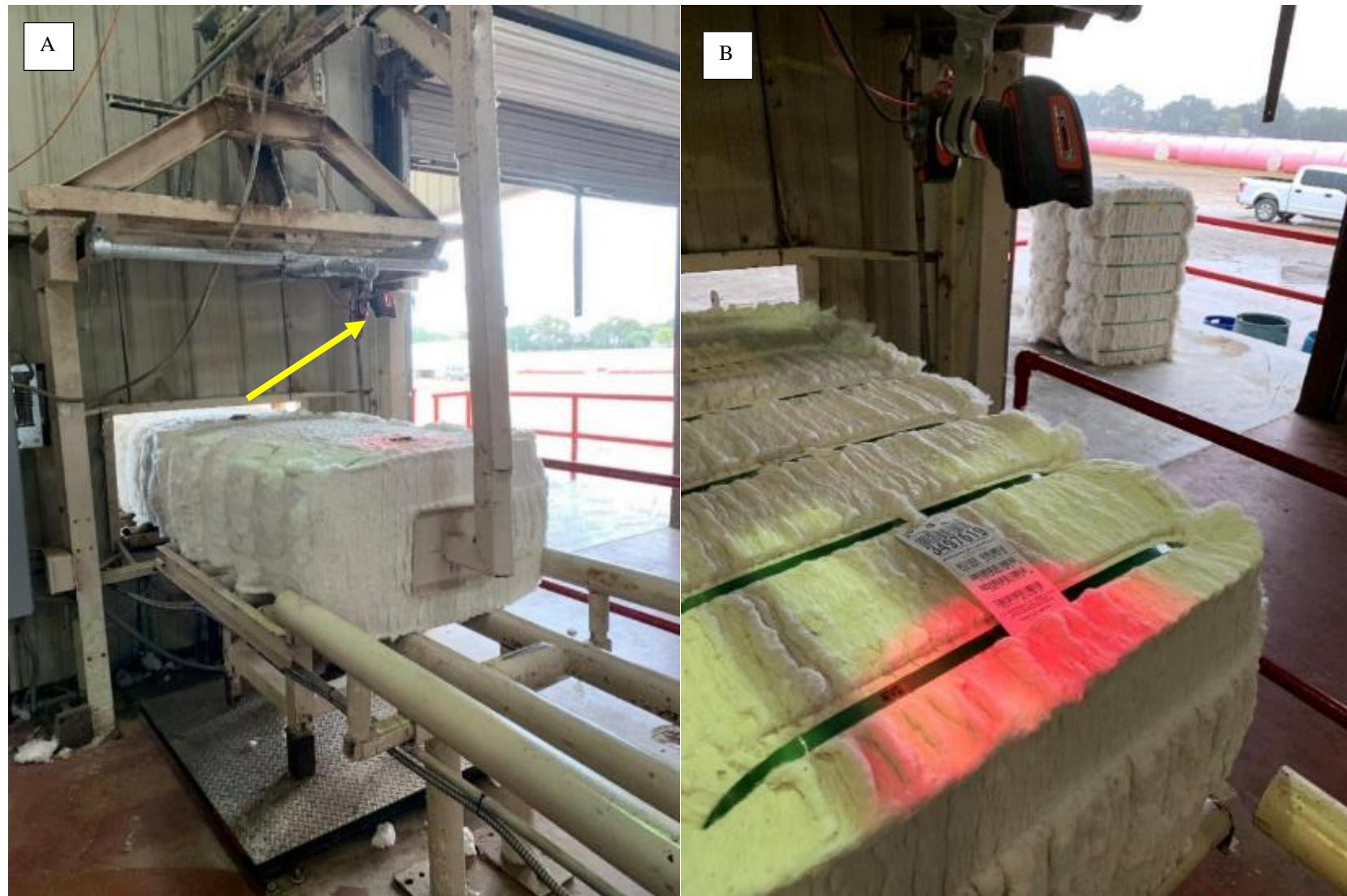
Figure 14. PBI Logger scanning system mounted above the bale scale. Bale PBI tags are scanned as the pusher moves the bale onto the scale (A). The width of the tag scanning zone is shown in pink on the end of the bale (B).
