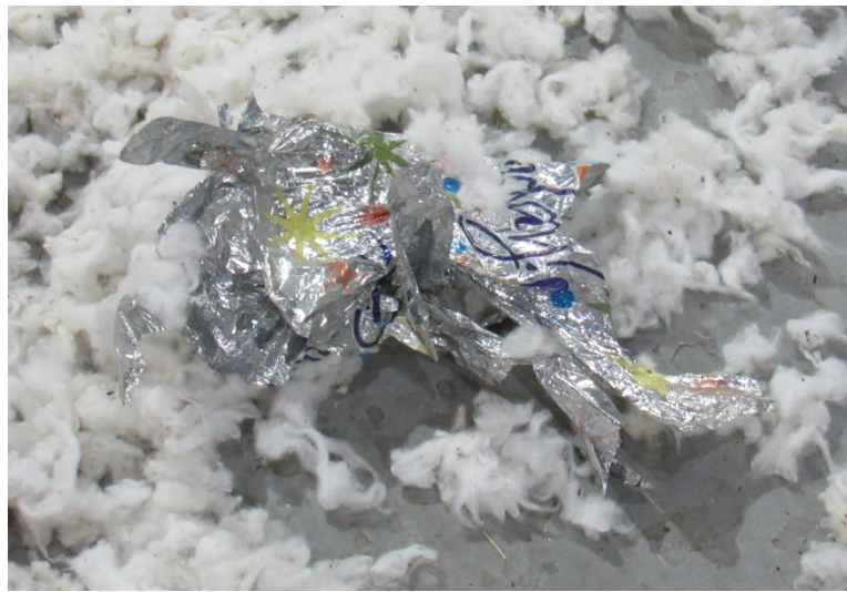
Figure 8. Mylar® balloon detected and ejected by the VIPR™ System.
