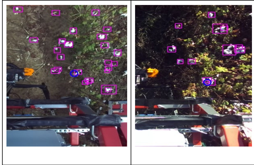
Figure 7. Boll detection using YOLOv3. Right when it was cloudy and left in direct sunlight.
