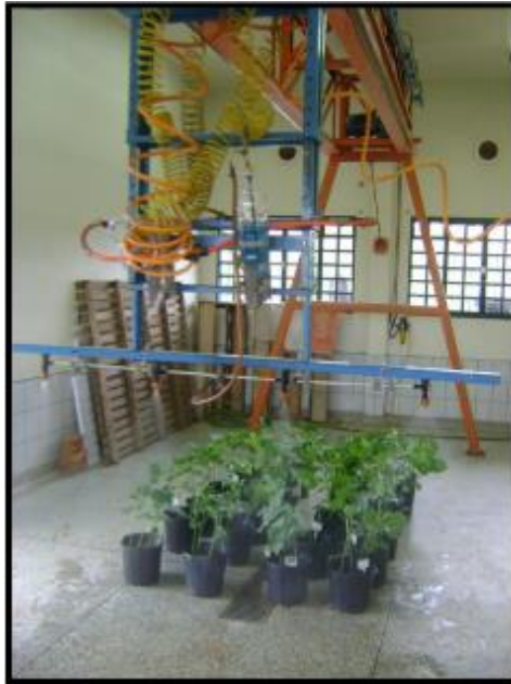
Figure 1. Stationary sprayer used for application of herbicide solution and rain simulation.
