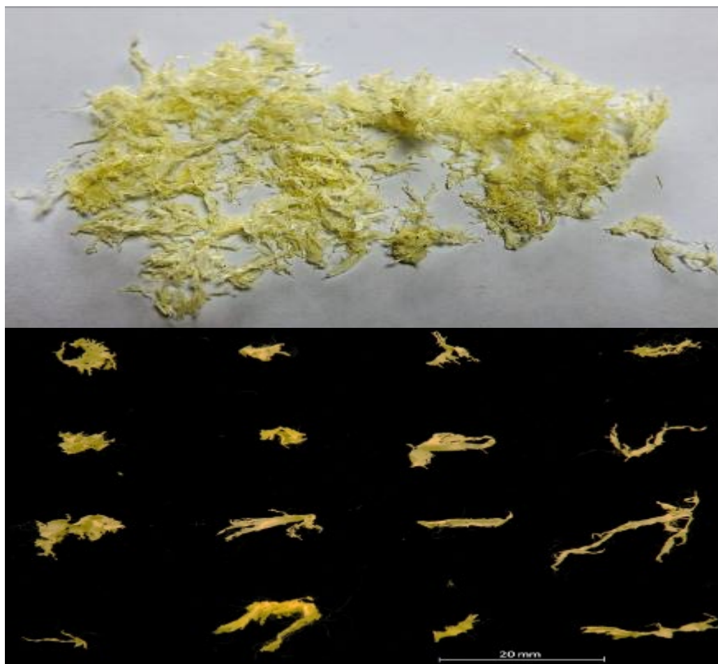
Figure 8 Examples of plastic wrap removed per card can of 9.2 kg.
