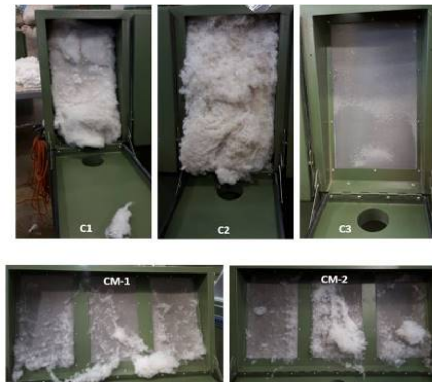
Figure 7 Image of impurities removed per card can of 9.2 kg.
