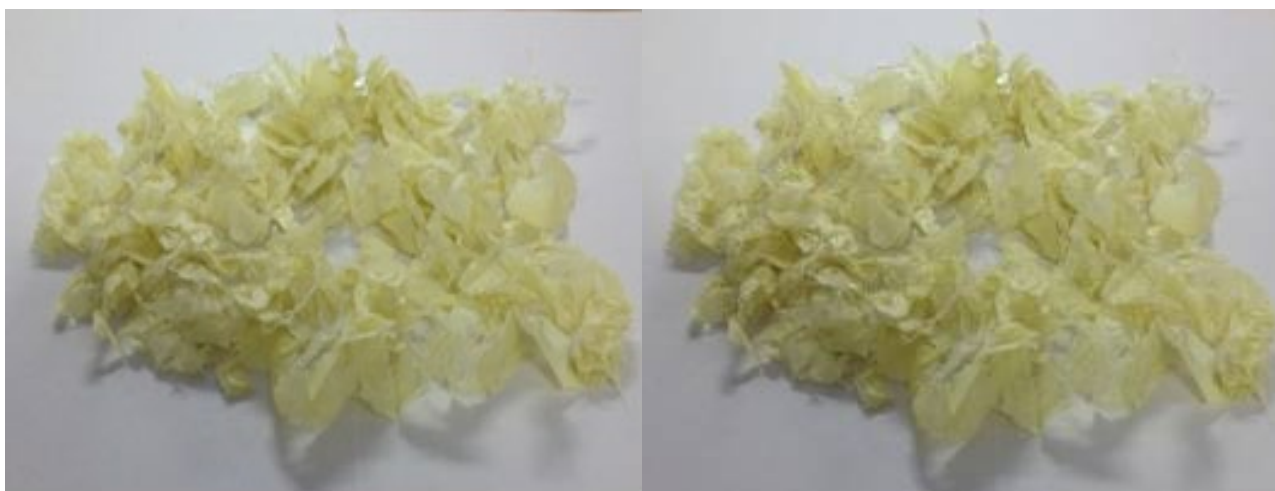
Figure 4 Six and eight grams of plastic wrap used to contaminate bales
