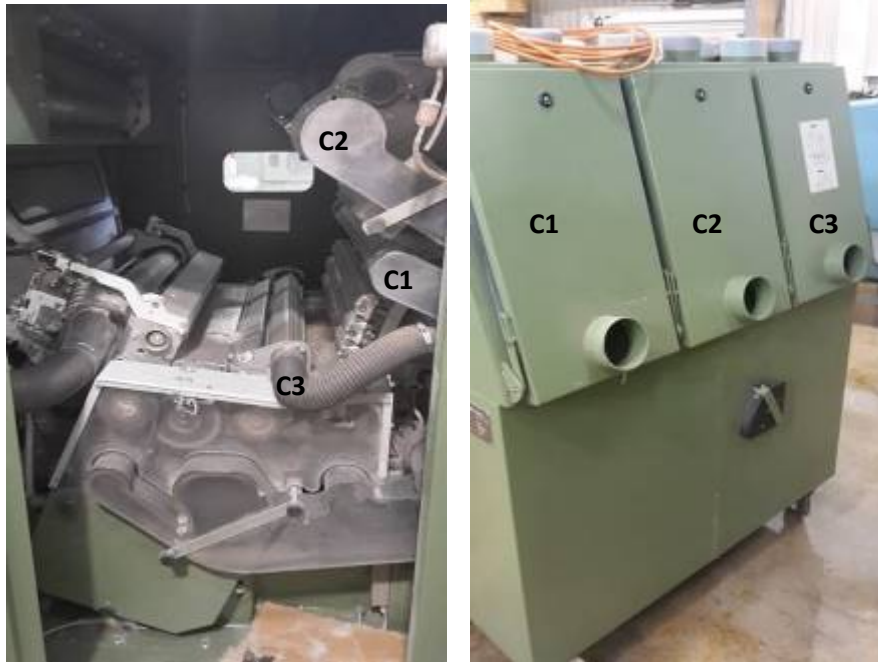
Figure 5 WAC connection to carding machine
