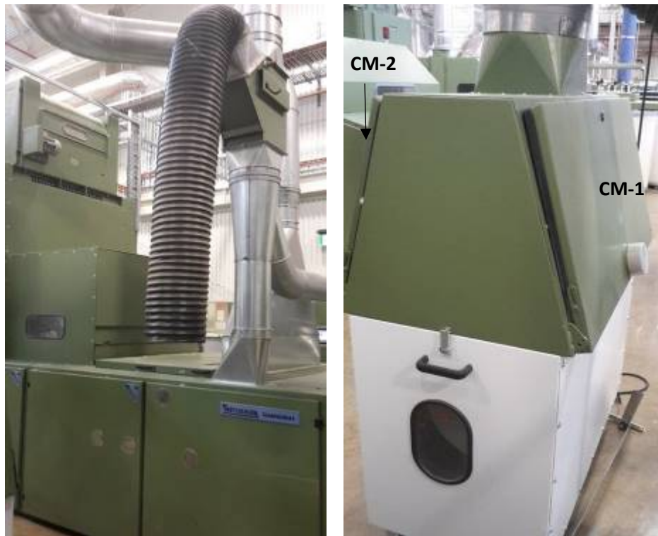
Figure 6 WAC connection to Cleanomat
