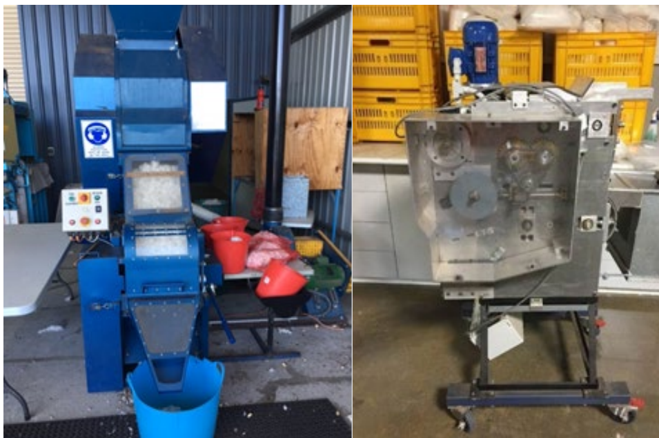
Figure 3. Image of sample gin and lint cleaner
