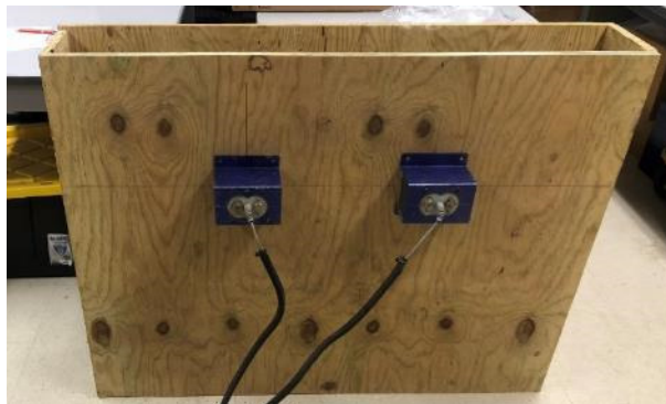
Figure 1. Sensors installation on the mimic duct for lab tests.
