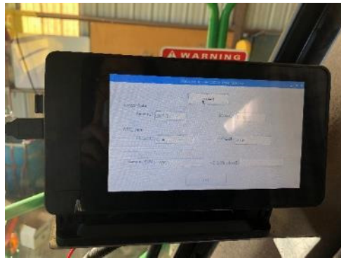
Figure 3. Data processing system location in the cab.
