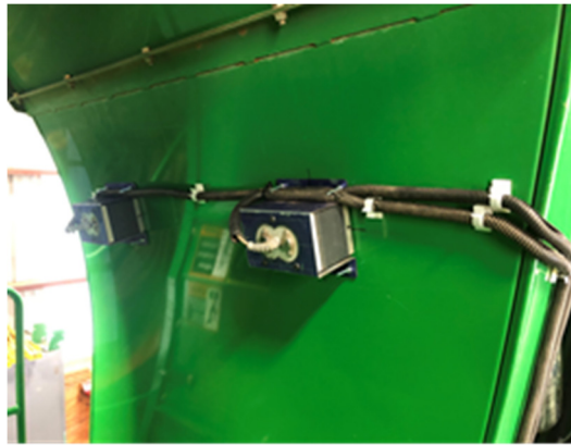
Figure 2. Sensors location on the cotton stripper 7460.
