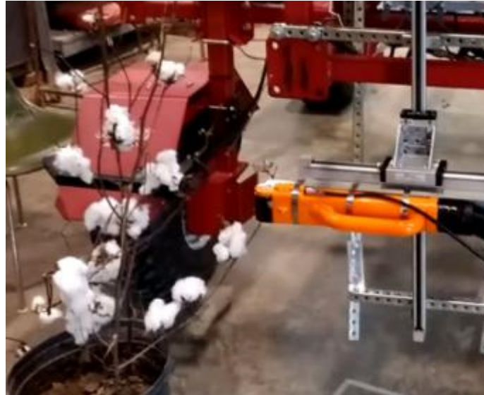
Figure 3. the end-effector comes close to the cotton bolls and sucks them using vacuum suction
