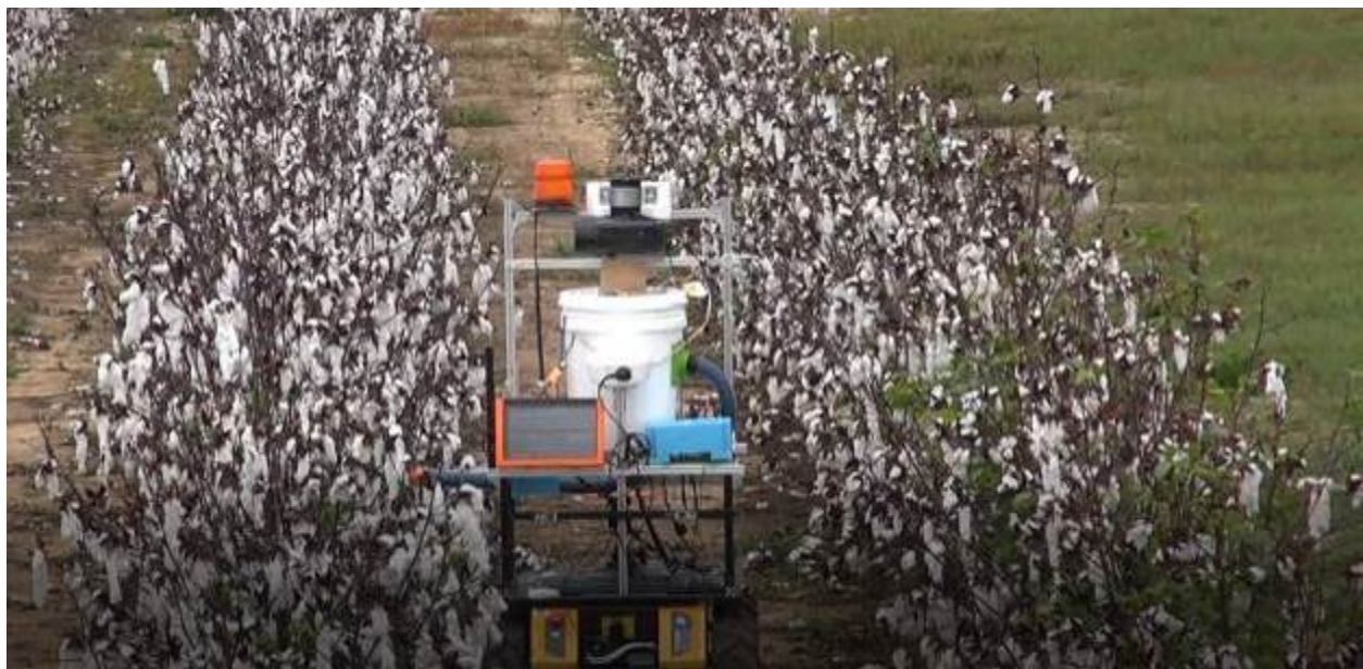
Figure 2. Clemson robot with harvest platform in skip row cotton field (76-inches between planted rows).
