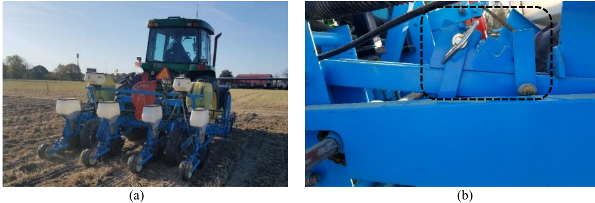
Figure 1. (a) 4-row Monosem NGPlus vacuum precision planter, and (b) downforce control assembly (spring-loaded arm and pin attachment shown in the dashed box) used for downforce adjustments in the study.
