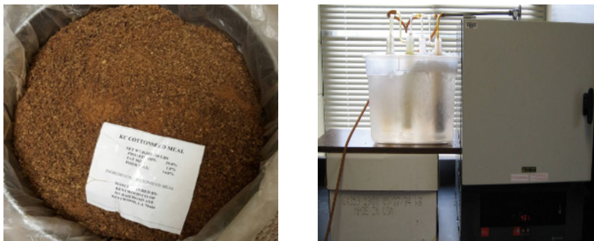
Fig. 1. Defatted cottonseed meal (left) and custom-made lab-scale slow pyrolysis system (right)
