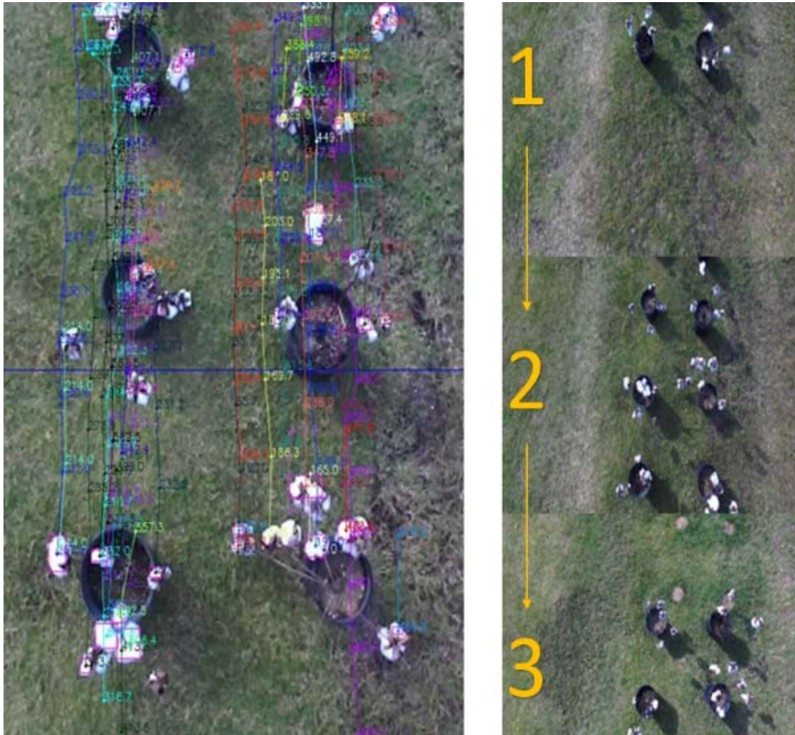
Figure 4. Left image show processed boll position and tracking of the boll while the right images show a series of 3 image frames acquired from the moving camera
