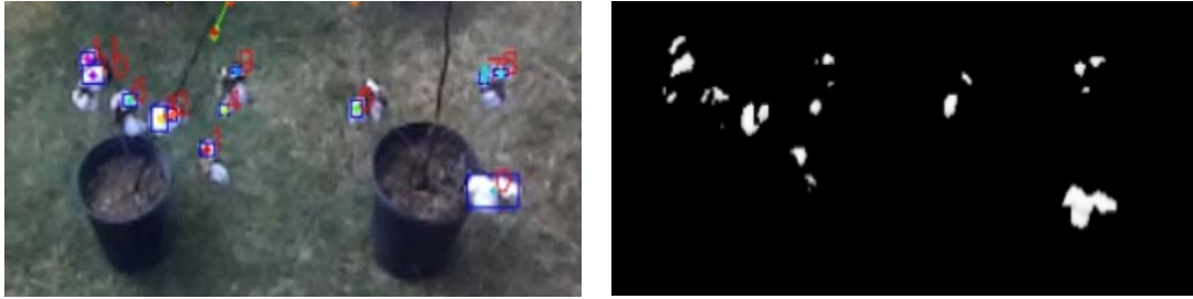
Figure 6. Comparing the contour detection. The larger the contour threshold the lower the number of bolls detected.
