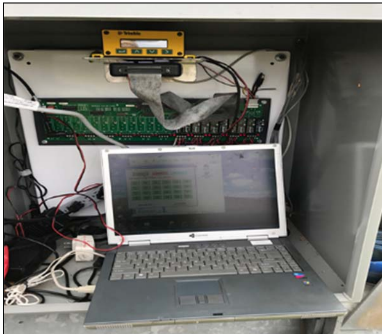
Figure 2: Variable-rate nitrogen control system (GPS receiver; control PC; and solid-state relay board).
