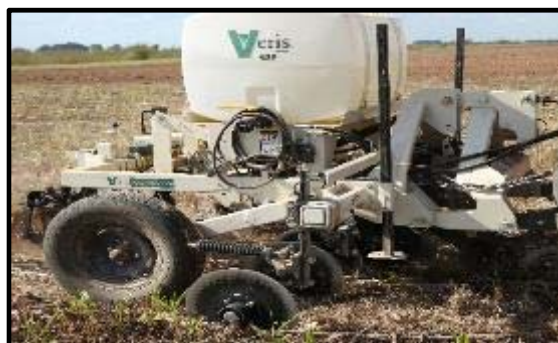
Image 1: Veris MSP3 being used in field operation to quantify continuous soil EC and color data and timed interval pH measurements.
