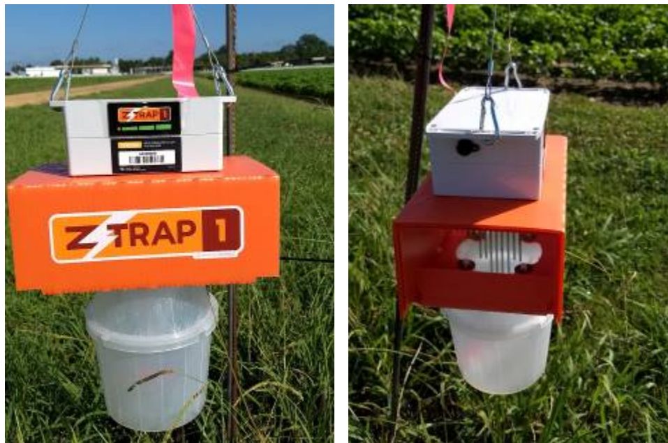
Fig. 1. Side and end view of the Z-trap used in this study
