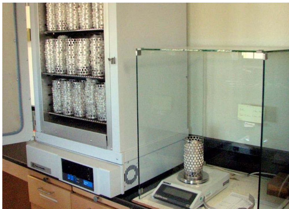
Figure 3. Determining dry weights adjacent to one of the high-capacity ovens.
