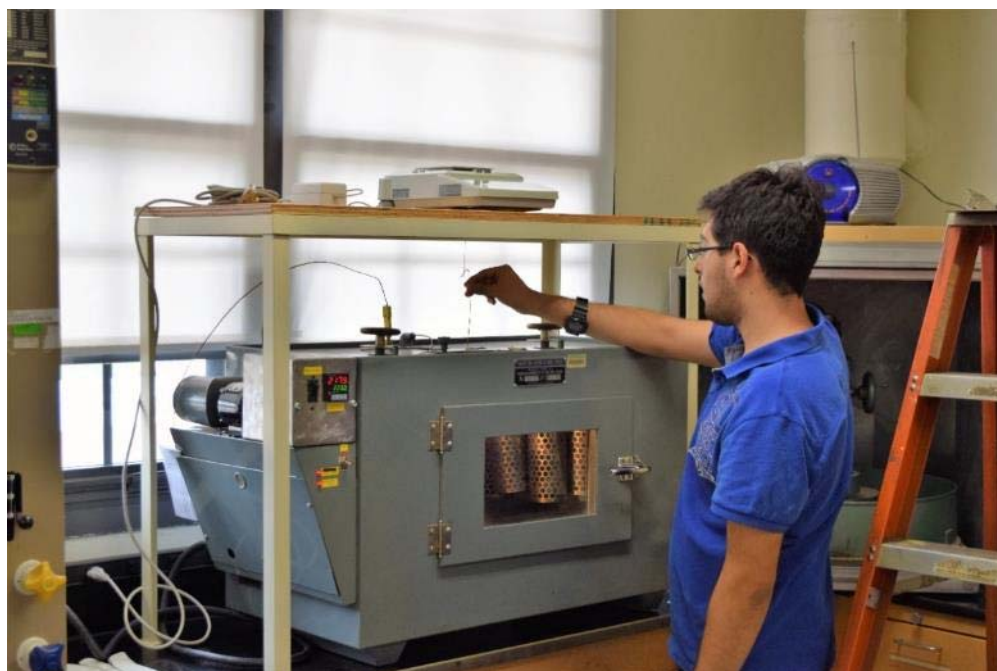
Figure 2. Determining dry weights inside one of the weighing ovens.
