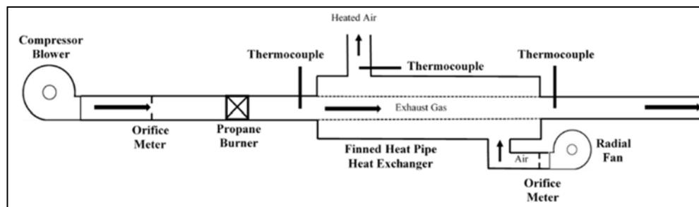
Figure 3. Set-up of heat exchanger experiments.
