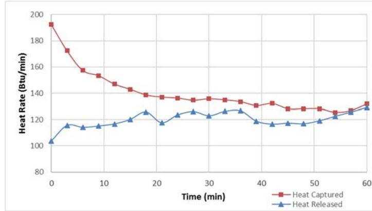
Figure 4. Heat rate results from an air flow rate of 75 cfm.
