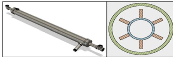
Figure 2. Final design of the finned HPHE (left) and sectional view of the inner pipe, outer pipe, and fins (right)
