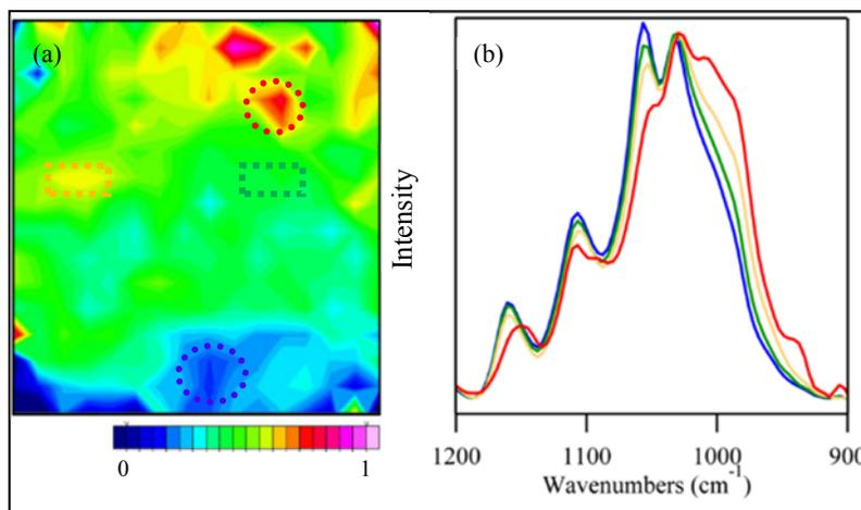
Figure 5. Chemical image for a cotton fiber bundle (20 DPA, STV 474), and FTIR spectra from the indicated sections of the map.
