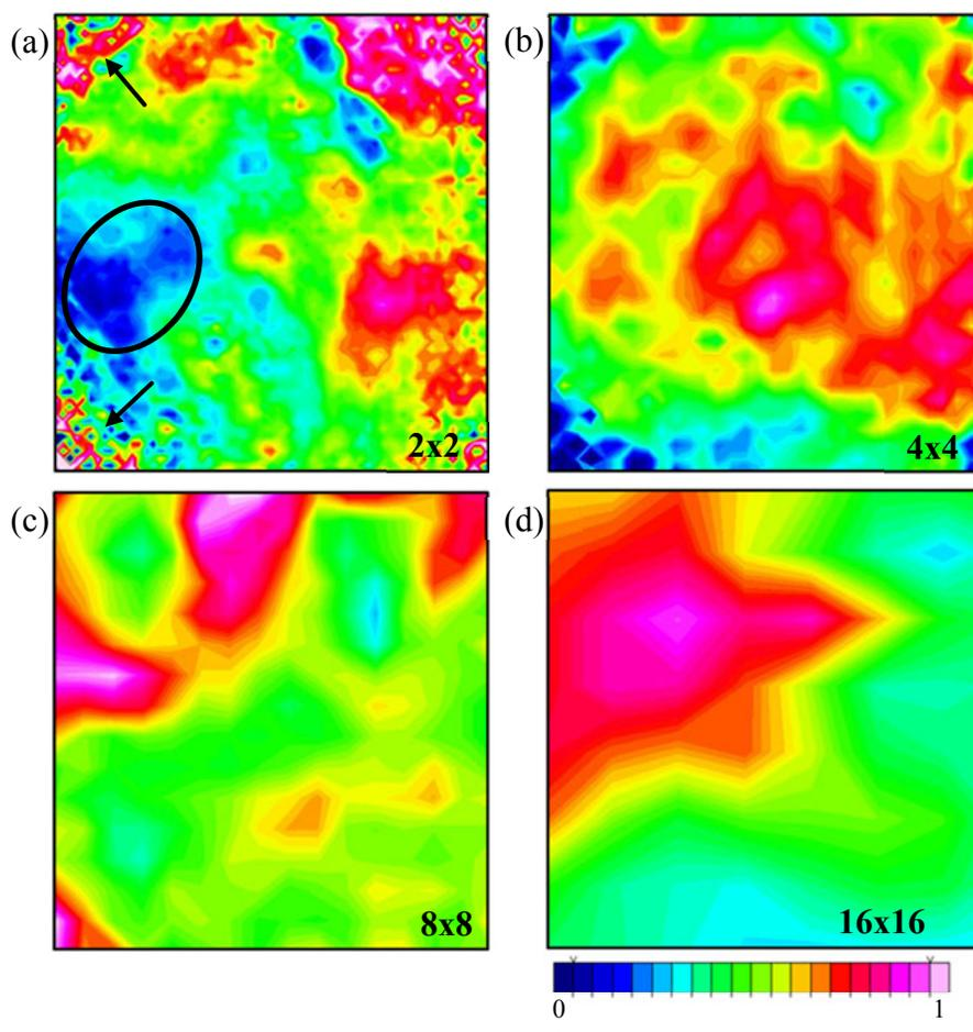
Figure 3. Chemical images for cotton fiber bundles as determined with a FTIR instrument equipped with a single reflection ATR accessory and a FPA Mid-IR detector. Images show data grouped into (a) 2x2, (b) 4x4, (c) 8x8, and (d) 16x16 pixels. Map tones reflect the integration intensity of the C-O bending region ( $1185\text{-}950\text{cm}^{-1}$ ).
