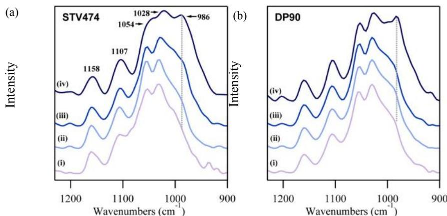
Figure 4. FTIR spectra of the C-O stretching region for cotton fibers harvested at different developmental time points. Spectra were collected utilizing a single reflection ATR attachment and a FPA detector. Two varieties were examined: (a) STV474 and (b) DP90. For each variety, 4 time points are shown: (i) 18 DPA, (ii) 20 DPA, (iii) 22 DPA, and (iv) mature fibers from open cotton bolls (+60 DPA). Indicated numbers are in wavenumbers.
