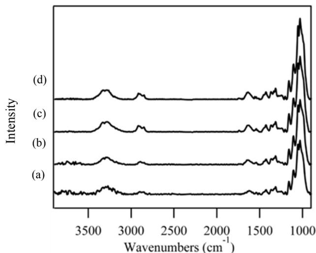
Figure 2. FTIR spectra of a cotton fiber bundle as determined with a single reflection ATR accessory and a FPA Mid-IR detector. Spectra were produced by grouping data into defined areas of (a) 2x2, (b) 4x4, (c) 8x8, and (d) 16x16 pixels. Spectra are the average of five sampling points, and are shown shifted along the y-axis (normalized absorbance).
