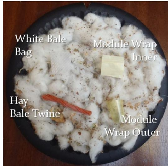
Figure 4. Example of contamination samples on seed cotton background prepared for hyperspectral imaging.
