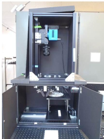
Figure 3. Short-wavelength infrared reflectance spectral imaging system.
