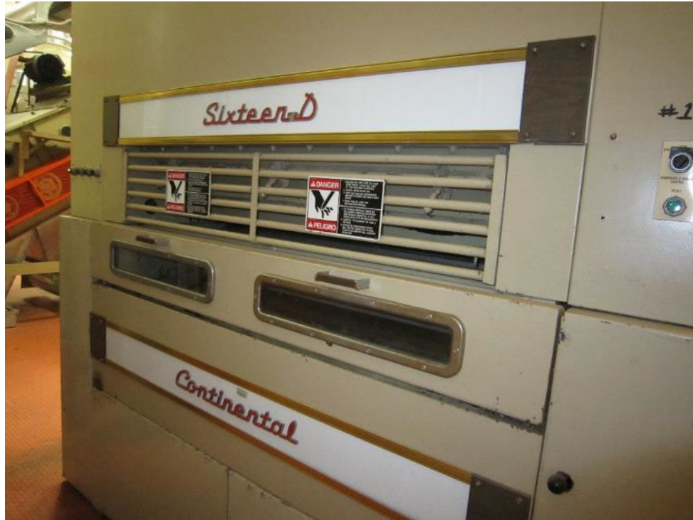
Figure 3. Continental SixteenD saw-type lint cleaner (STLC) used in this work.
