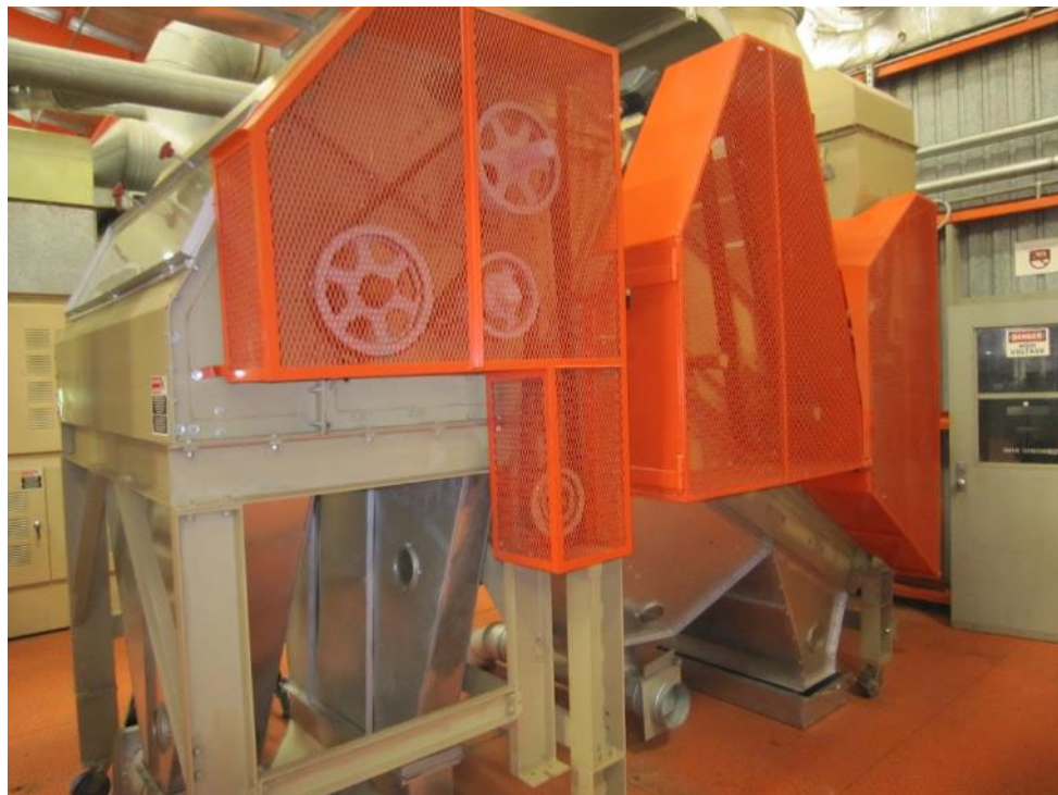
Figure 4. Experimental cylinder and saw lint cleaner (CSLC) used in this work.
