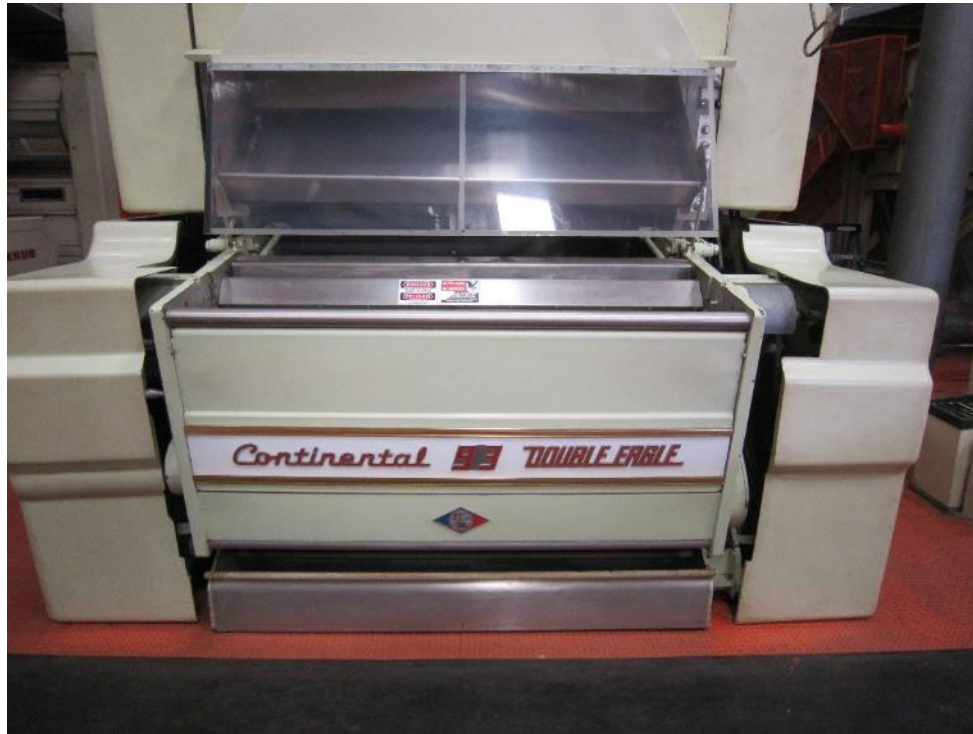
Figure 1. Saw type Continental Double Eagle gin stand used in the work.
