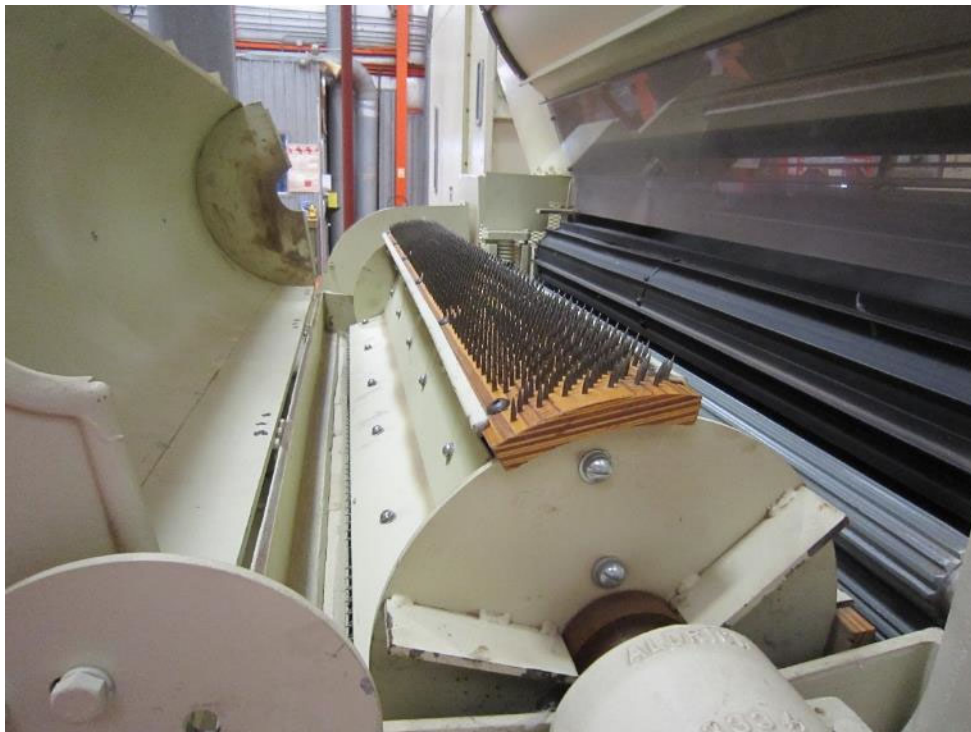
Figure 6. The Kirschner beater portion of the ALC used in the work.
