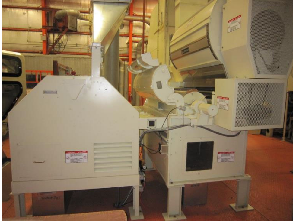
Figure 5. The entire ALC lint cleaner with the Kirschner beater portion on the right and the air-jet portion on the left of the photograph.
