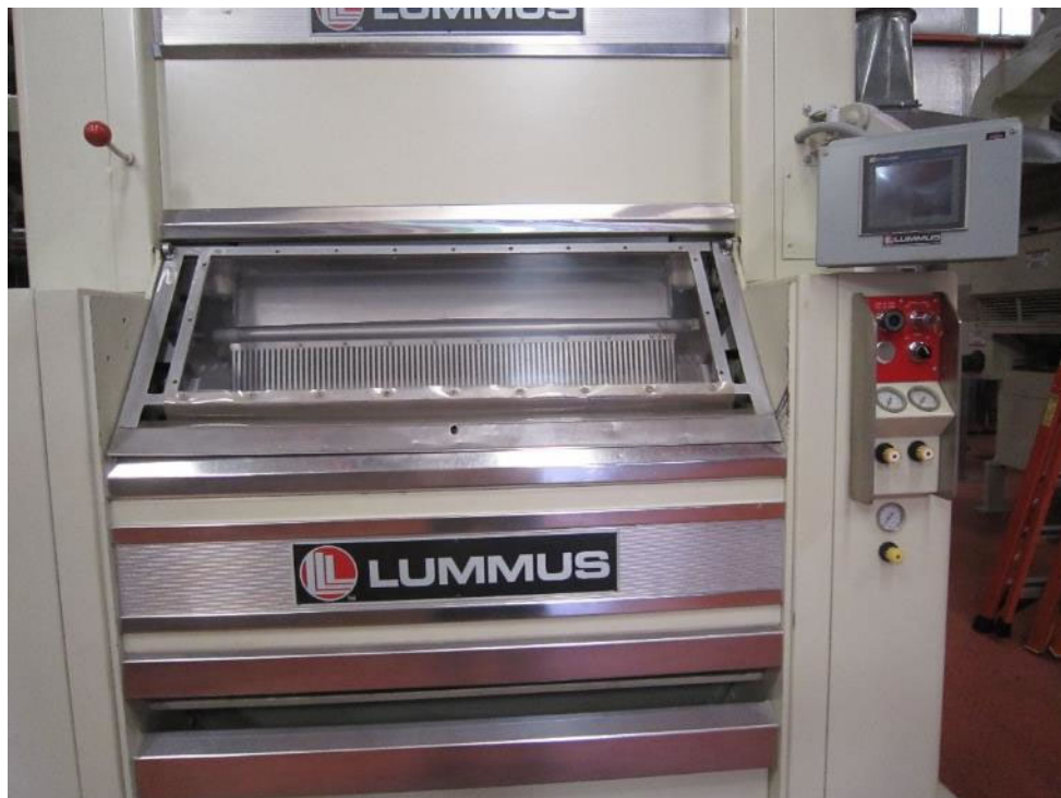
Figure 2. Lummus high-speed roller gin stand (HSRG) used in the work.
