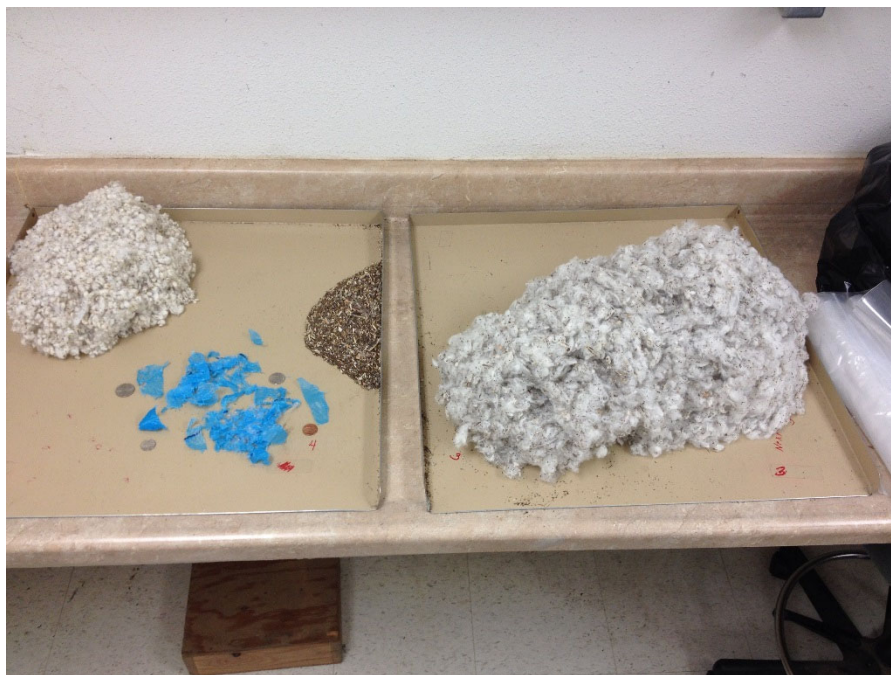
Figure 2. Plastic removed in seed cotton cleaning waste.
