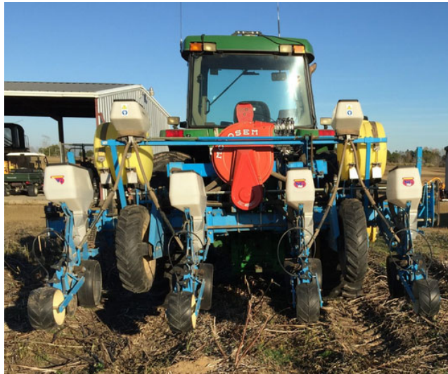
Figure 1. Four row (36 in. wide) Monosem planter used for planting the cotton.
