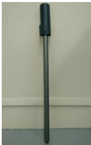
Figure 2. AquaCheck capacitance probe.
