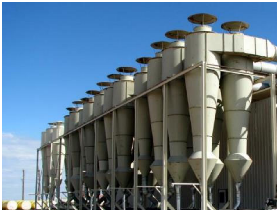
Figure 1. The particulate emissions abatement device used by the US cotton ginning industry is the 1D3D cyclone; this example installation shows the fully enhanced version with modified inlets and expansion chambers.
