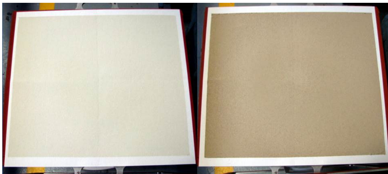
Figure 4. The filter at left was from a run with an inlet velocity of 1600 feet per minute, and the filter at right from a run with an inlet velocity of 3200 feet per minute. Both runs presented the cyclone with 800 grams of trash.
