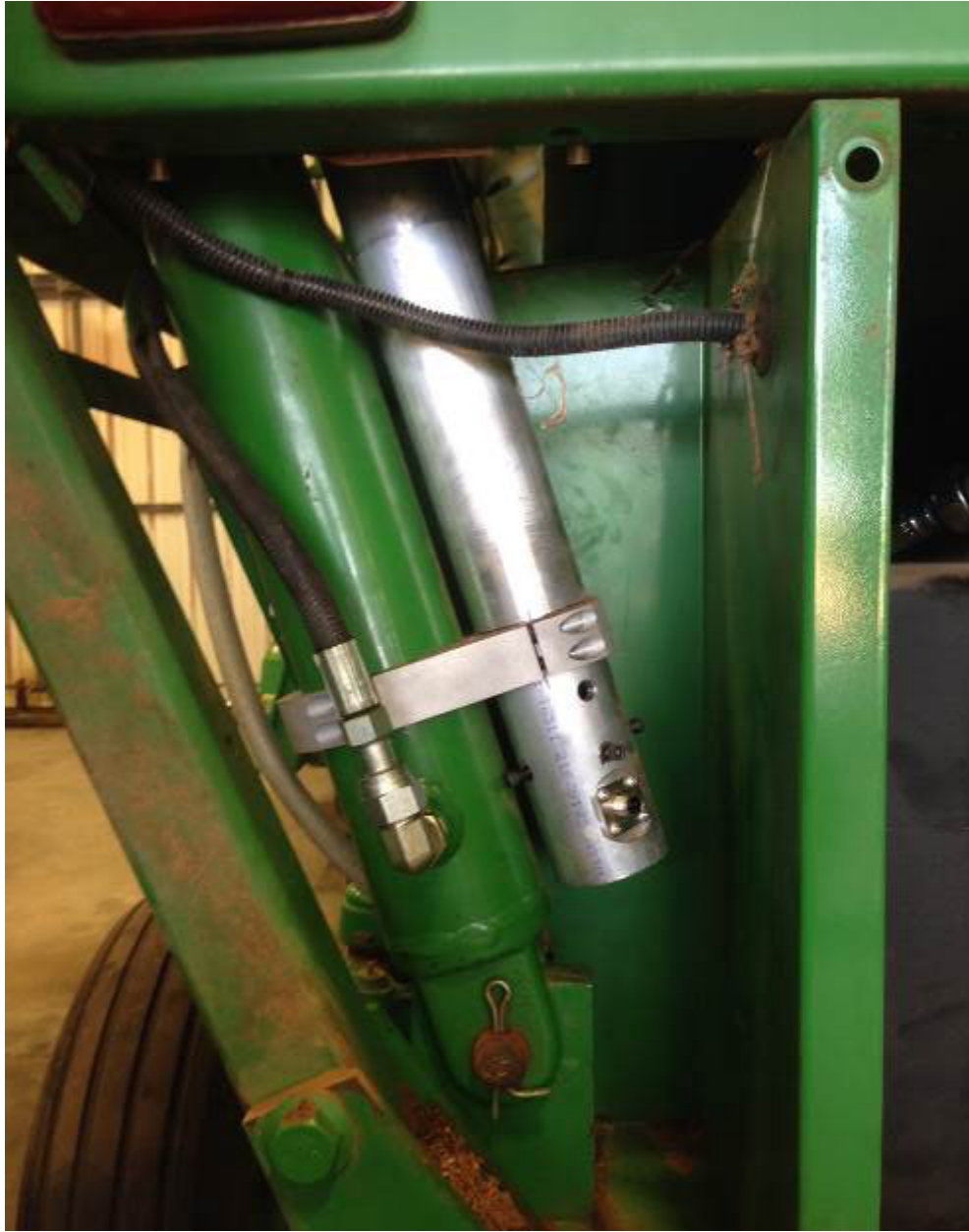
Figure 10. Image of the linear position transducer follower assembly housing mounted to the rear basket lift cylinder.
