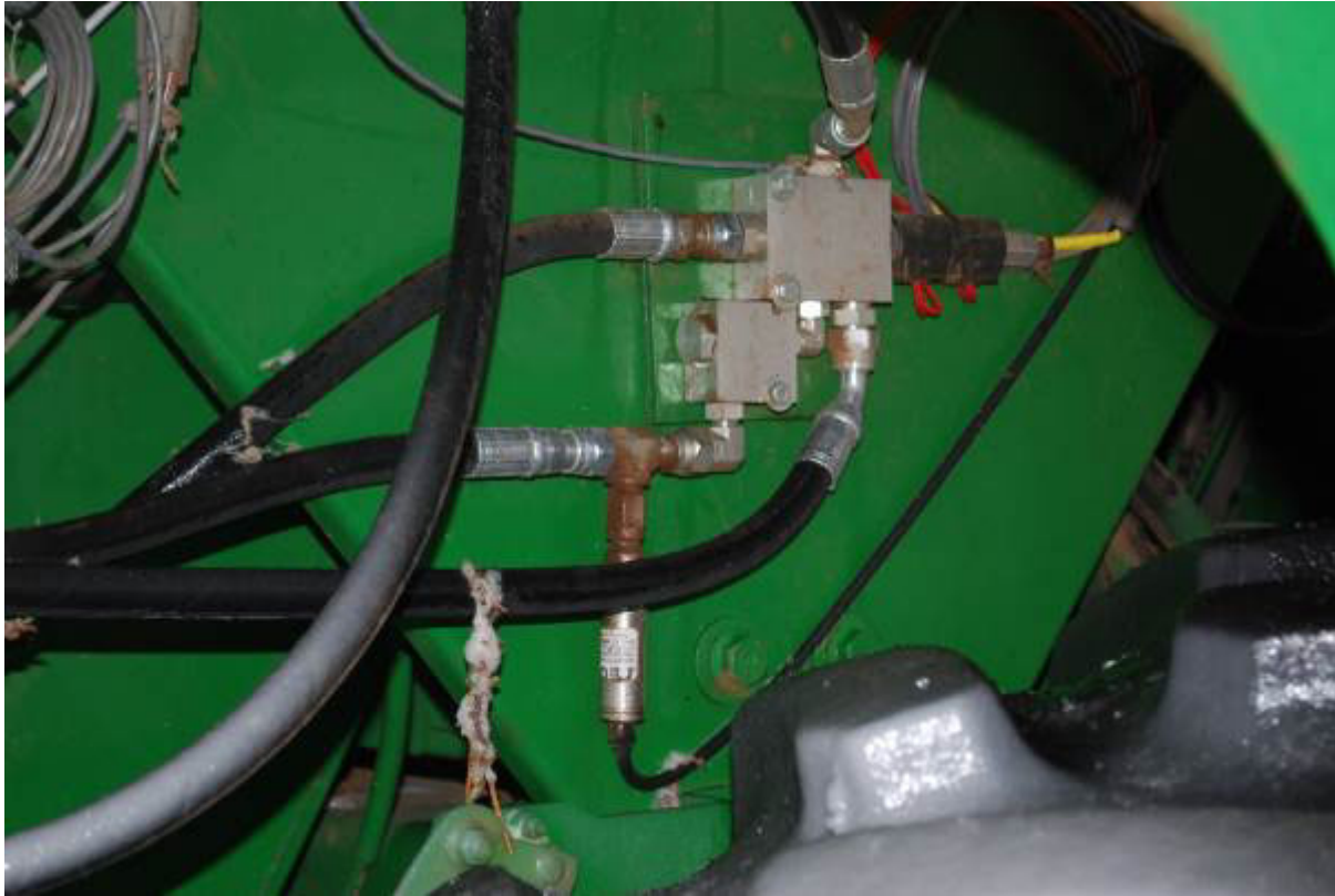
Figure 8. Hydraulic PWM valve (top) used to raise the basket and pressure transducer (bottom) used to measure lift cylinder circuit hydraulic pressure.
