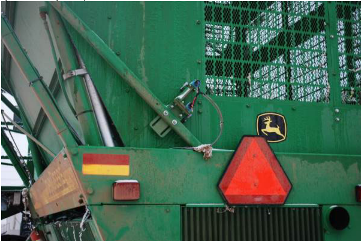
Figure 9. Limit switches mounted at the rear of the basket used to slow and stop the movement of the basket.
