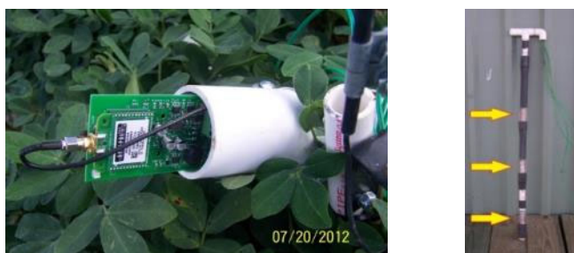
Figure 1. The electronic components of the UGA SSA node are presented in the photo to the left. They include the main board which is connected with the three Watermarks® sensors and the radio board. The black wire connects the radio board with the antenna. The photo at the right shows a UGA SSA probe with the three Watermarks® soil moisture sensors. The probe can be easily installed after planting and extracted prior to harvest.
